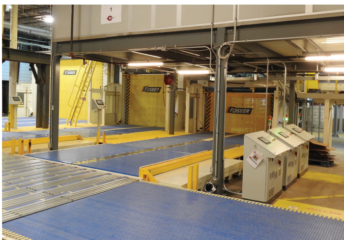
No fork lifts are needed to move containerboard from the Foster corrugator to Acme Corrugated’s converting machines.
