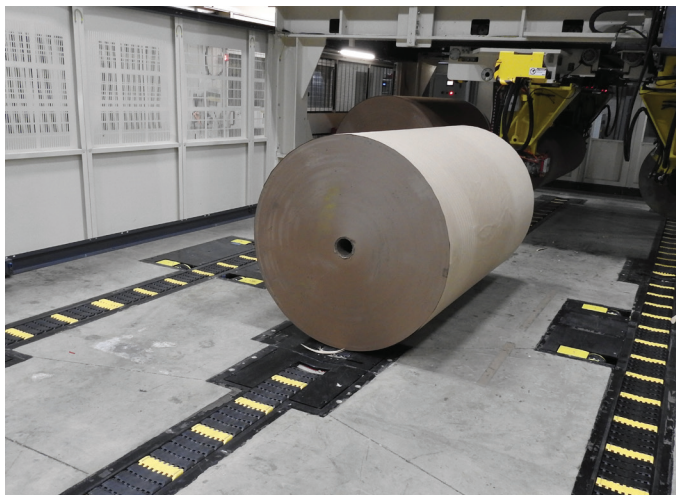
Paper rolls are inserted into the singlefacer via a cradle and material handling system by Harmax.
